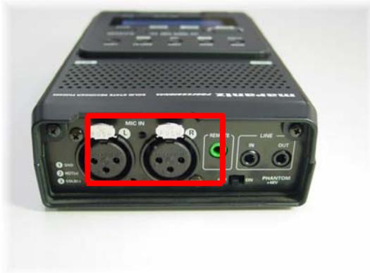
The microphone inputs are placed at the back (red border), what can be impractical (for example working with stereo-microphones and 3,5/ 6,35 mm connectors).
